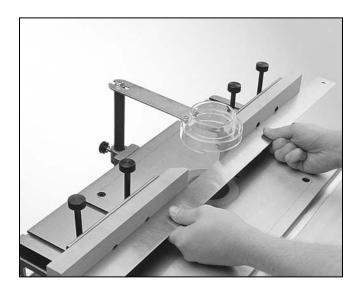
Figure 18. Fence alignment.
